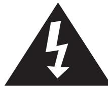
The lightning flash with arrowhead symbol, within an equilateral triangle, is intended to alert the user to the presence of uninsulated dangerous voltage within the product's enclosure that may be of sufficient magnitude to constitute a risk of electric shock to persons.
