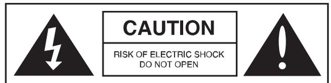
**WARNING:** TO PREVENT FIRE OR SHOCK HAZARD, DO NOT EXPOSE THIS APPLIANCE TO RAIN OR MOISTURE. THE APPLIANCE SHALL NOT BE EXPOSED TO DRIPPING OR SPLASHING. NO OBJECTS FILLED WITH LIQUIDS SHALL BE PLACED ON THE APPLIANCE.
